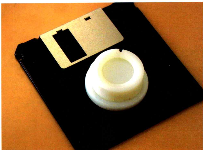
Device for Diffusive Gradient in Thin film (DGT) technique
