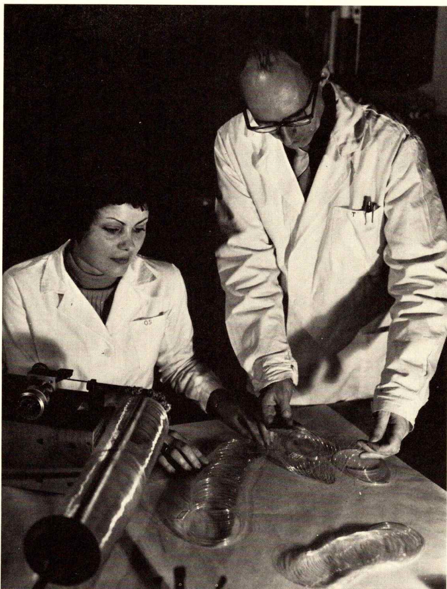
Fig. 8. Drawing of special glass capillary columns in the apparatus constructed in the Institute according to the design of Dr. K. Tesařík: The efficiency of columns reaches up to 7000 theoretical plates per metre (Dr. K. Tesařík, O. Smolová).
