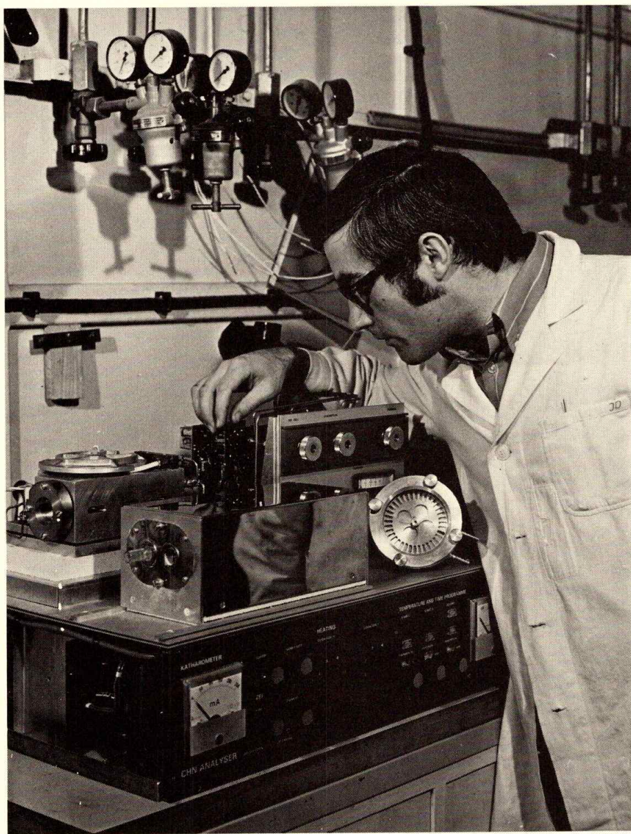
Fig. 10. Functional tests of a CHN-1 elemental analyzer. The instrument, for which Czechoslovakia gained the agreement on specialization within COMECON countries, is manufactured by Laboratory Instruments, N.E., Prague, according to the patent of the staff member Vlastimil Rezl. The instrument was awarded the diploma of the international exhibition INTERLAB in Ostrava in 1971, the Golden Medal at the International Engineering Trade Fair in Brno in 1973 and the prize of the Czechoslovak Academy of Sciences in 1975 (J. Drozd).
