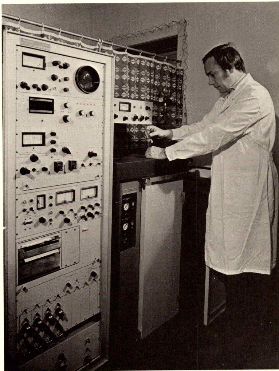
Fig. 13. Injection of the sample under analysis into a gas chromatograph combined with a mass spectrometer. The instrument permits the analysis of very complicated mixtures and reliable identification of their components (L. Keprt).
