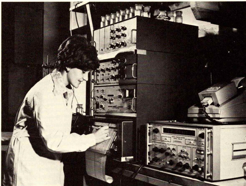
Fig. 12. Determination of trace amounts of atmospheric pollutants by gas chromatography using the method of frontal chromatographic concentration. Evaluation of the chromatogram — quantitative determination by means of an electronic digital integrator (M. Roudná).
