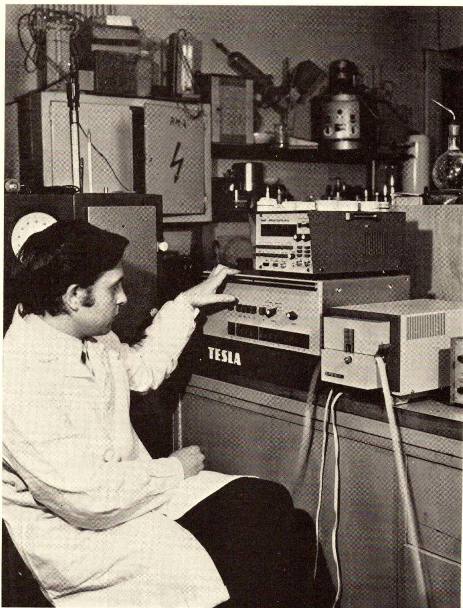
Fig. 14. Automatic processing of chromatograms in a JPR 12 minicomputer. The instrument serves as a control element for an automatic petrochemical laboratory (Ing. O. Bártů).
